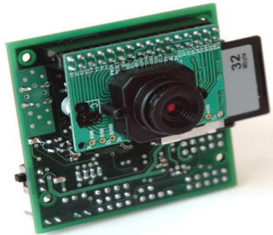
Figure 2. CMUCam3: Main board, sensor and an MMC memory card for mass storage
