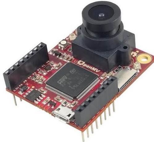
Figure 6. OpenMV's main board
