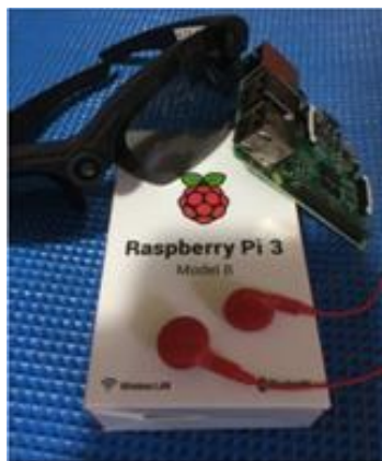
Figure 1. Hardware components of the proposed computer vision system: the Raspberry Pi 3 Model B board, the videoglasses with the camera, an earphone
