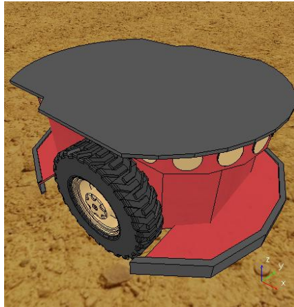
Figure 2. MP Pioneer P3-DX, created in the simulation environment V-REP PRO EDU
