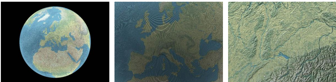
Figure 6. From left to right: Zoom into a 3D point cloud of earth data with 1 billion points (file size is 42.2 GB)
